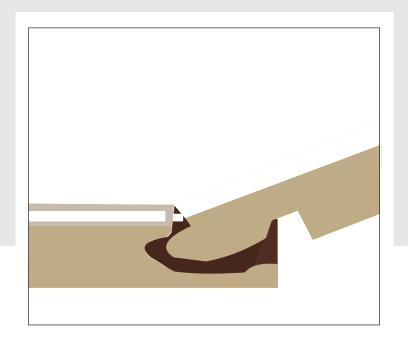
Our Click-N-Lock<sup>®</sup> Tiles come with Wel-Lock<sup>™</sup> technology, a unique locking mechanism that obviates the need for glue or cement.
