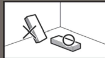
In case any visual faults are detected on materials, do not install the faulty products and contact your local dealer, to obtain information about the way of proceeding.
